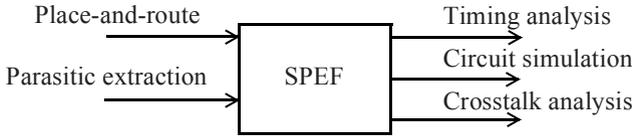
**Figure C-1** *SPEF is a tool exchange medium.*
