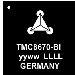
Figure 32: TMC8670-BI device marking
